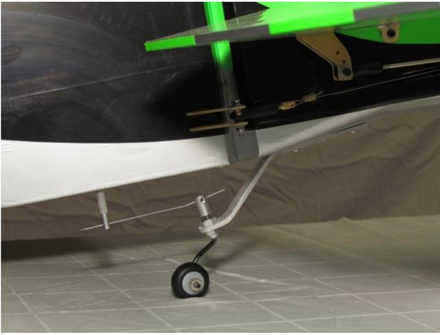
Drill bottom of rudder to accept steering pin.
