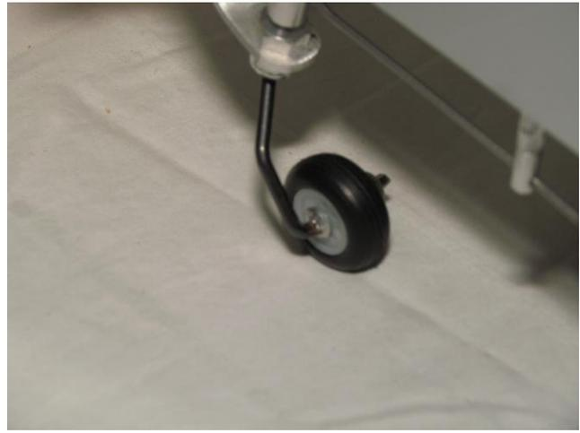
Washer was soldered on to center the wheel on
