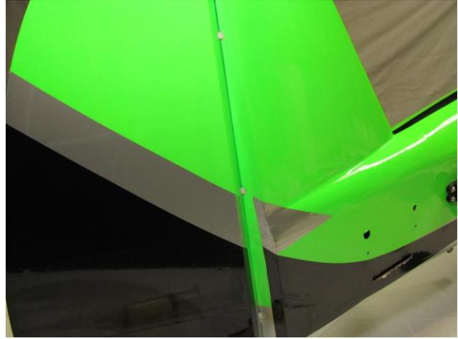
Once all hinges have been installed, clean off excess adhesive. Flex hinge back and forth to help align the hinges in the holes. Rudder hinges have been completed. Note: minimal hinge gap and throw is bevel to bevel. If necessary, increase gap slightly to achieve full control surface throw.
