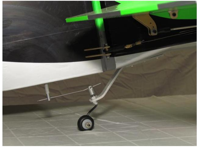
Prepare pull-pull cables. Measure distance between ball link on rudder horn and ball link on servo arm. This can be done by inserting a balsa stick (anything that will fit) through the cable outlet hole to the ball link on the servo. Be sure to cross from one side to the other. Add  $\frac{1}{2}$ " to allow for  $\frac{1}{4}$ " thread into each ball link.
