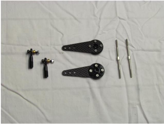
Prepare servo arms. Carbon fiber arms are provided for all control surface servos. The round wheels that come with the servos can be used. If desired, aluminum wheels can be purchased from RedWing RC for an additional cost. These wheels are drilled and tapped to fit the arms. We will be using the short turnbuckle pushrods for ailerons.
