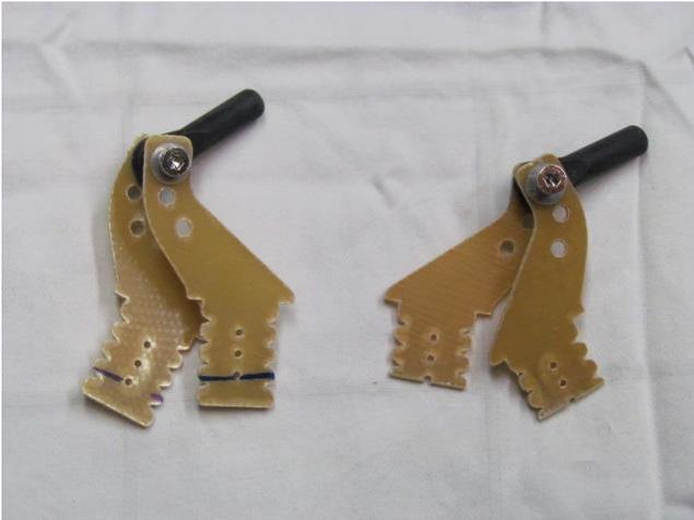
Rudder uses two pairs of control horns for pull-pull cables. The horns install directly opposed from each other, thus will not fit unless trimmed. The horns on the left have been marked. The horns on the right have been trimmed. Verify both sets of horns fit prior to gluing in place.
