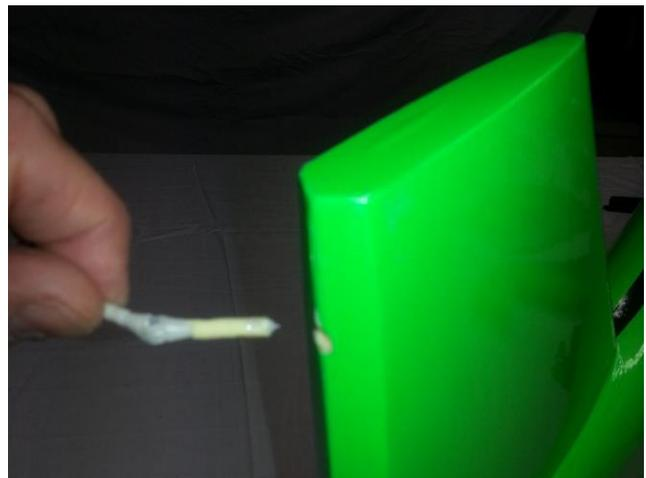
Inject a small amount of adhesive into the hole in the flying surface. Also add some adhesive to the barbs of the hinge. Insert the hinge into the hole until the pin is at the hinge line.
