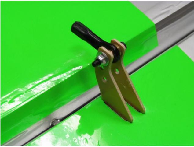
Assemble aileron control horns and tighten bolt. Scuff bottom of control horns (glue area) with coarse sandpaper for better adhesion. Inject epoxy into both control horn slots. Apply additional epoxy to both sides of each control horn. Insert control horns into slots and clean up excess epoxy that oozes out of slots.
