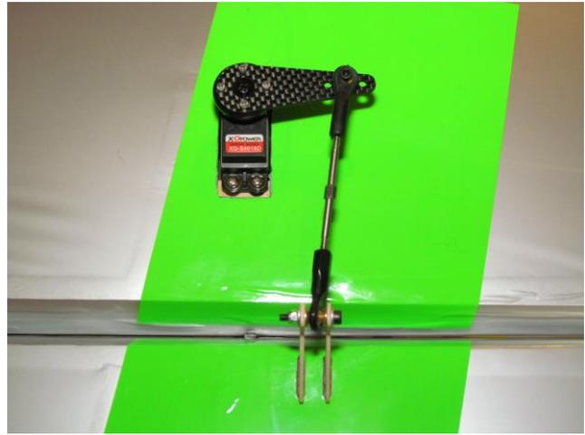
Verify servo is centered. Install control arm on servo. Servo arm should be parallel to hinge line. Manually center the aileron. Hold turnbuckle pushrod up to the two ball links to see how far the turnbuckle has to be threaded into each ball link. Thread turnbuckle into ball links. Note: the turnbuckle has left hand and right hand threads.
