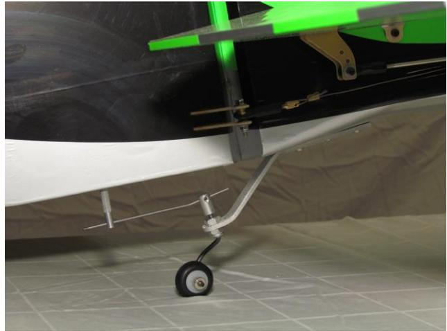
Install tail wheel bracket only. Note: wheel and steering linkage will be installed later.
