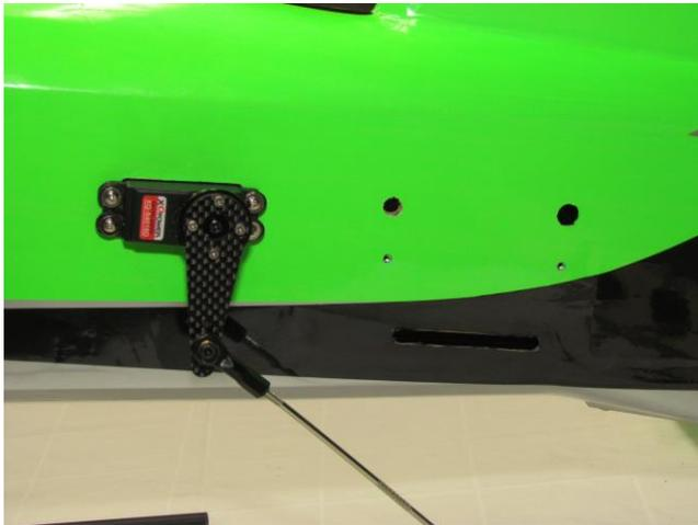
Install elevator servo with a 24" heavy duty extension. Servo spline is closer to the rudder. Be sure to restrain the connector on the extension. Temporarily install servo arm and turnbuckle pushrod. Longer turnbuckles are used on elevator linkages.
