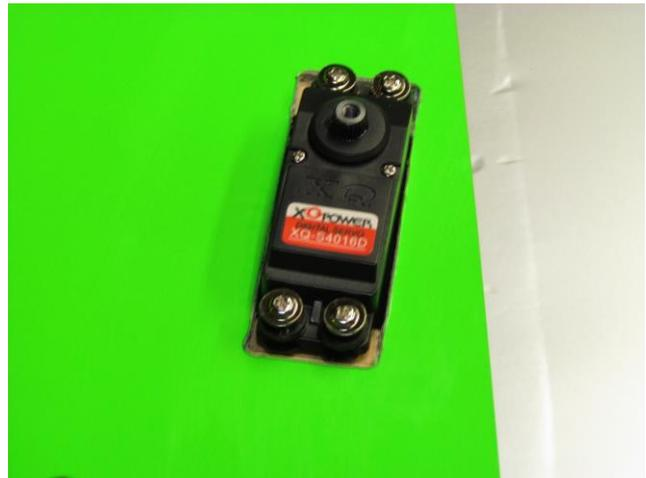
Install aileron servo. Note: servo spline is closer to the leading edge of the wing.
