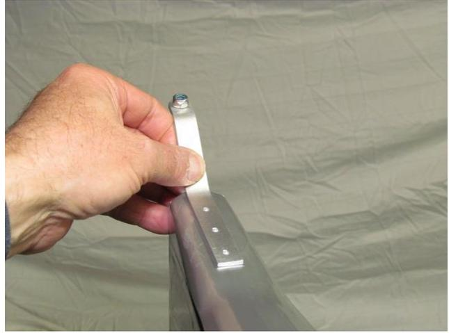
Place tail wheel bracket in positions and mark location of the mounting holes. Note: locate the bracket as low as possible on the tapered section at the back of the fuselage. Location shown is too high and will result in difficulty when setting up tail wheel steering. It was actually installed about 3/4" lower.
