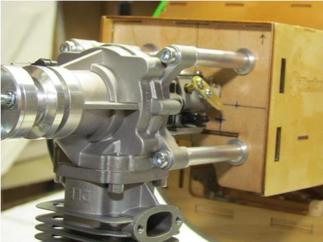
Install standoffs using thread lock on bolts. Note: a 10 mm open end wrench fits on the flats of the standoffs. Temporarily mount engine. Mark locations of throttle linkage and fuel line on firewall.
