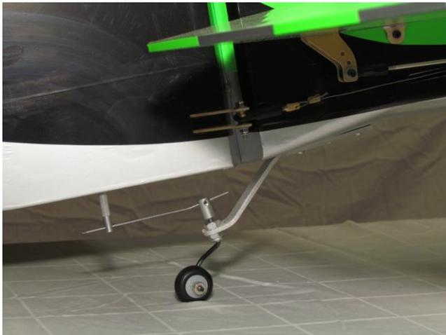
Thread one end of cable onto ball link on rudder horn. Feed cable through fuselage to rudder servo arm.
