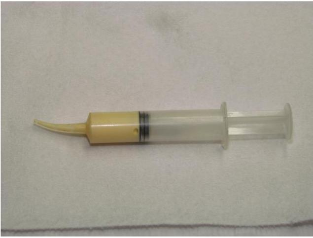
Several different types of adhesive are acceptable for installing hinges. Epoxy, Gorilla Glue and aliphatic resin (Titebond II) all work. One benefit of the aliphatic resin is it cleans up with water until it cures. A dental syringe is an excellent tool for injecting glue into the holes.
