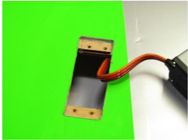
Set aileron servo in position. Drill all four holes for mounting screws. Install screws, then remove and move servo out of the way. Place a drop of thin CA glue in each hole to toughen threads in the plywood.
