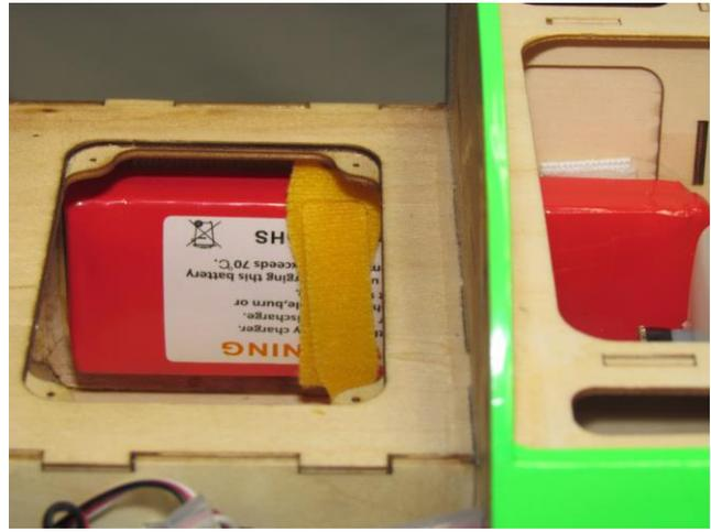
A 3000 mah LiFe battery (available from RedWing RC) is being used for both the radio and ignition. It is held in place with a couple of strips of Velcro and a strap that goes through the motorbox side and around the battery. Verify sheet metal screws used for attaching cover over access hatch don't hit the battery.
