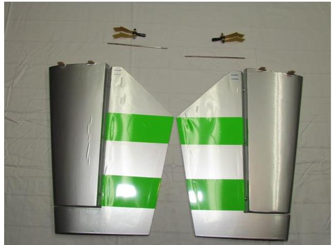
Slots for elevator control horns have been marked, but not cut yet.
