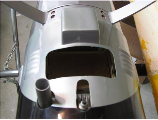
Enlarge holes per revised marks. This time smooth edges, etc. Hole for spark plug includes ignition cap.
