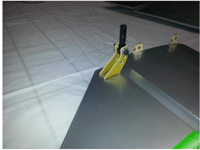
Elevator control horns have been installed. Note: excess epoxy has not been cleaned off yet.
