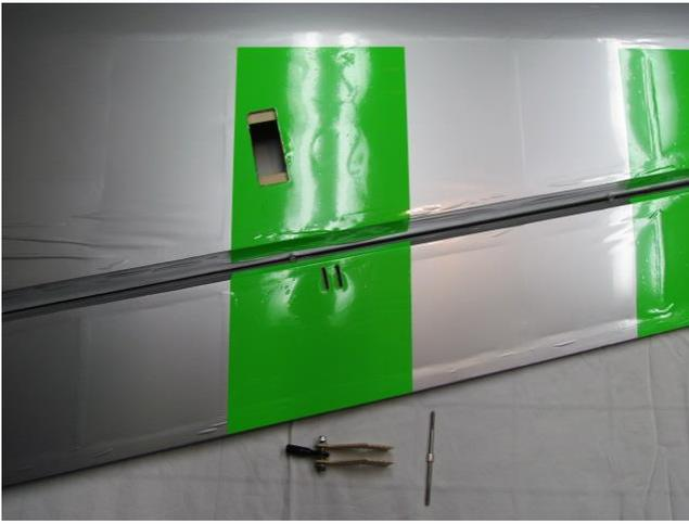
Remove covering over aileron servo openings and control horn slots. Covering can be removed by either cutting it off with an X-acto or similar knife or by melting it with a pencil type of soldering iron. The soldering pencil seals the covering to the structure, but leaves some excess that needs to be cut off.
